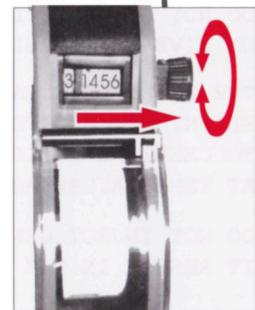
PULL OR PUSH THE DIAL SHAFT TO THE DESIRED BAND AND ROTATE THE SHAFT IN EITHER DIRECTION. WHEN BANDS ARE SET. PUSH THE DIAL SHAFT INWARD.
