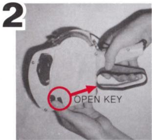
PULL BACK "BASE PLATE OPEN KEY" ON BOTH SIDES LIKE ARROW TO OPEN BASE PLATE AND PLATE COVER.
